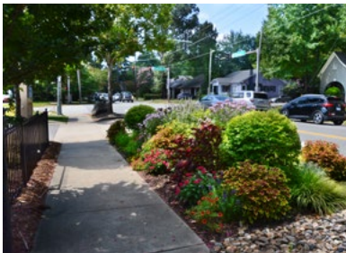
This buffer, landscaped with plants and rocks, also serves to absorb stormwater.
